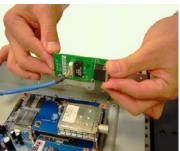
3. Disconnect the cable from the ethernet board.
