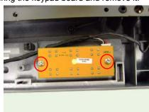
**3.** Remove the two screws securing the IR board, and remove the two screws securing the power button board.
