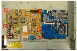
3. Remove the two screw, three short nuts, and four long nuts securing the D-tuner board.
