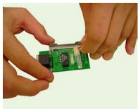
4. Remove the two screws securing the ethernet bracket and remove the bracket.
