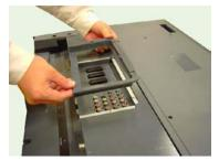
3. Remove the 20 screws securing the I/O bracket.
