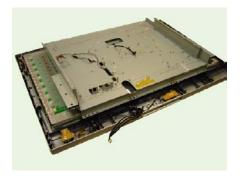
2. Remove the two screws securing the keypad board and remove it.
